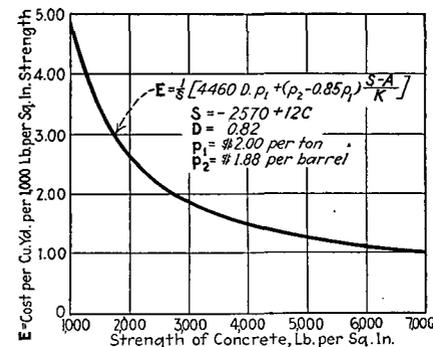
Fig. 3—Cost of concrete per unit of strength (1,000 lb. per sq.in.) decreases rapidly with an increase in concrete strength.
