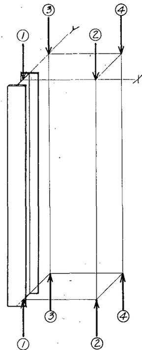
FIG. 1 VARIOUS LOAD POSITIONS APPLIED TO I-SECTION COLUMNS
